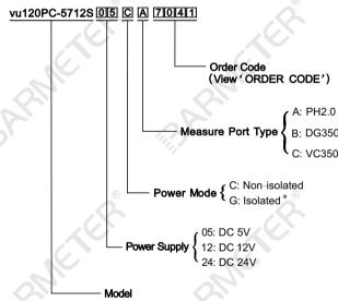
When choose isolated power mode, signal's unbalanced input(Pin 1 and Pin 2 are common ground) cannot be used.
